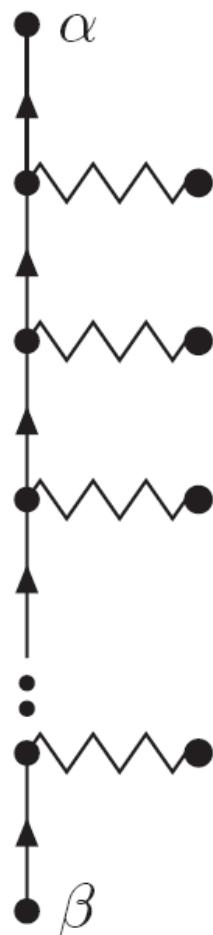
**Rule 1** Draw a directed line with  $k$  zigzag (horizontal) interaction lines  $V$  and  $k + 1$  directed unperturbed propagators  $G^{(0)}$
